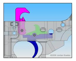
The end result is that the user of a semi-automatic firearm can fire rapidly by means of repeated use of the trigger. Critically, use of the trigger necessarily corresponds one-to-one with bullets fired. That is, a single pull of the trigger results in a single bullet fired. Without resetting the trigger, the disconnector cannot reset the hammer to the fully cocked position. And
