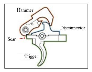
The trigger is the interface between the gun's internal mechanism and the human finger. The sear is the trigger's top-forward geometric plane, which locks snugly into a groove near the spring of the hammer. The hammer is the spring-loaded element that strikes the firing pin, causing ignition of the
